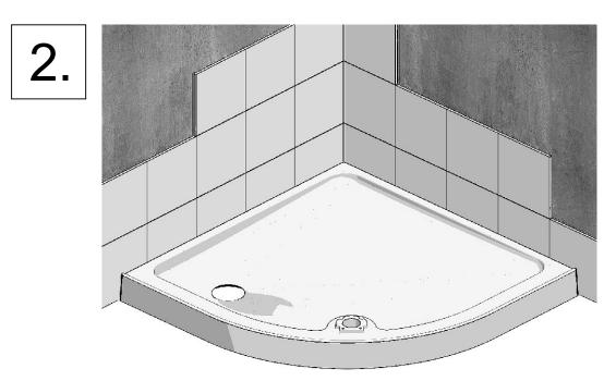
On picture 2 you have a tray external, in this case you can have the adjustment of 3mm.
